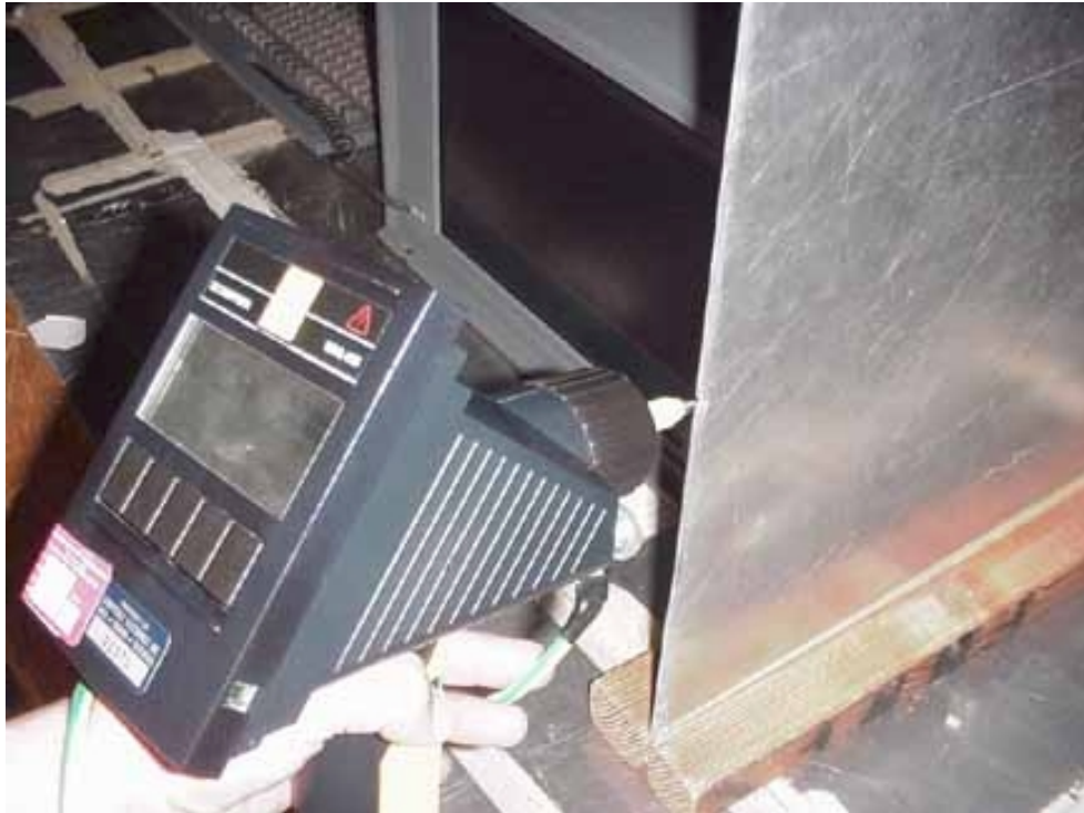
PHOTOGRAPH OF THE TEST SETUP FOR INDIRECT ELECTROSTATIC DISCHARGE TEST (VERTICAL COUPLING PLANE)
