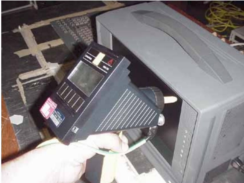
PHOTOGRAPH OF THE TEST SETUP FOR DIRECT ELECTROSTATIC DISCHARGE TEST (AIR DISCHARGE)
